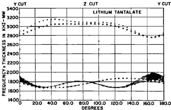
FIG. 6. Frequency constants of the fundamental resonances and antiresonances of a LiTaO<sub>3</sub> plate rotated around the X axis (rotated F-cut).
