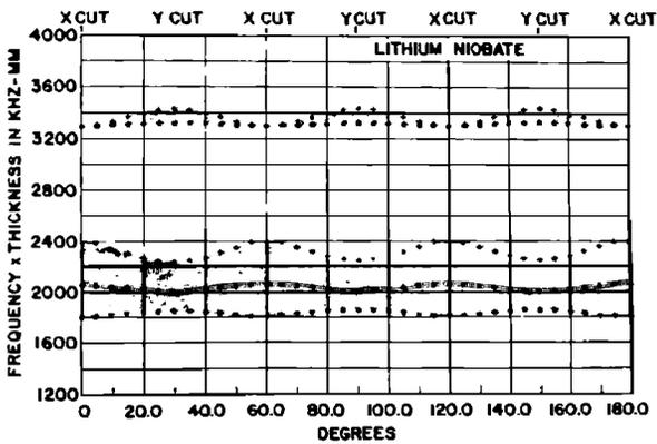
FIG. 12. Frequency constants of the fundamental resonances and antiresonances of a LiNbO<sub>3</sub> plate rotated around the Z axis.
