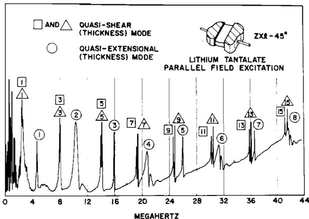
FIG. 1. Frequency spectrum of a rotated plate of lithium tantalate.
