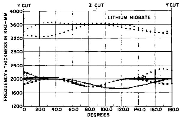
FIG. 10. Frequency constants of the fundamental resonances and antiresonances of a  $\text{LiNbO}_3$  plate rotated around the X axis (rotated F-cut).
