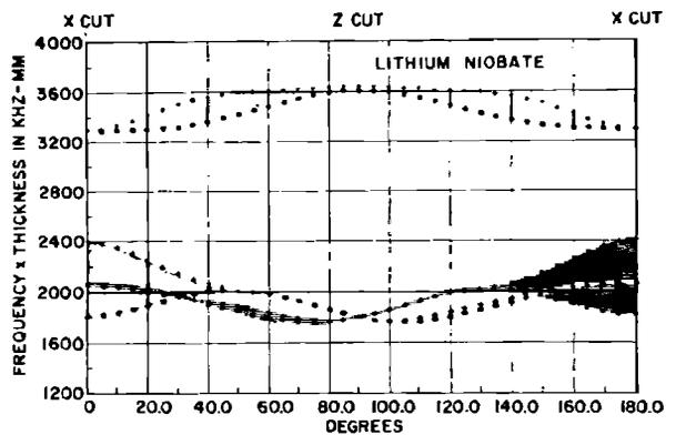
FIG. 11. Frequency constants of the fundamental resonances and antiresonances of a  $\text{LiNbO}_3$  plate rotated around the Y axis.
