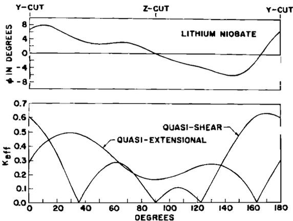
FIG. 13. Effective coupling factors and angle  $\phi$  between quasi-extensional wave displacement and plate normal for rotated Y-cuts of LiNbO<sub>3</sub>.
