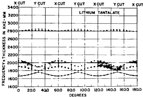
FIG. 8. Frequency constants of the fundamental resonances and antiresonances of a  $\text{LiTaO}_3$  plate rotated around the Z axis.
