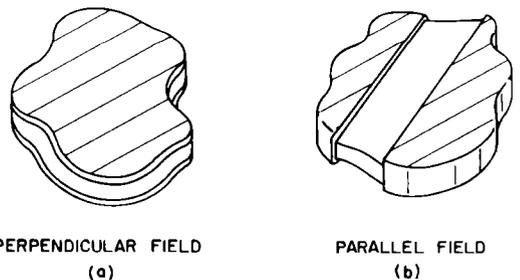
FIG. 4. Electrode configurations for (a) a perpendicular-field excitation, and (b) a parallel-field excitation.
