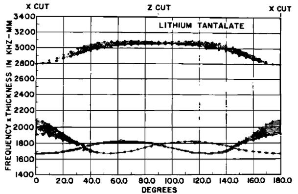
FIG. 7. Frequency constants of the fundamental resonances and antiresonances of a LiTaO<sub>3</sub> plate rotated around the Y axis.
