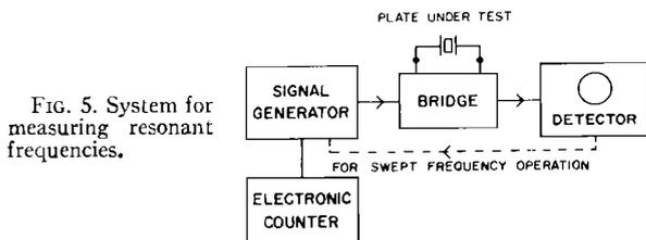
FIG. 5. System for measuring resonant frequencies.
