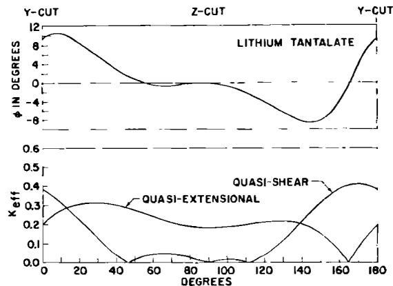
FIG. 9. Effective coupling factors and angle  $\varphi$  between quasi-extensional wave displacement and plate normal for rotated F-cuts of  $\text{LiTaO}_3$ .
